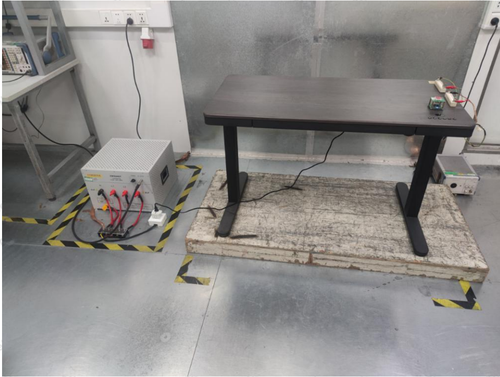
Photo of Conducted Emission Measurement
