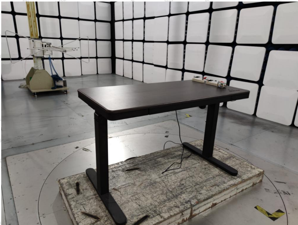
Photo of Radiation Emission Test
