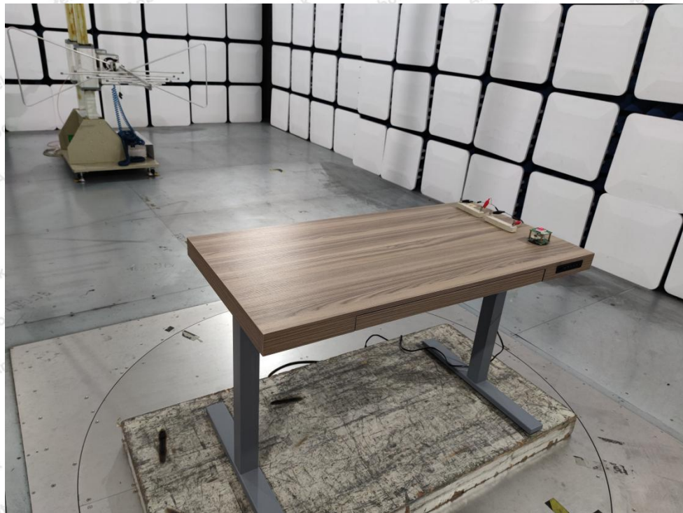
Photo of Radiation Emission Test
