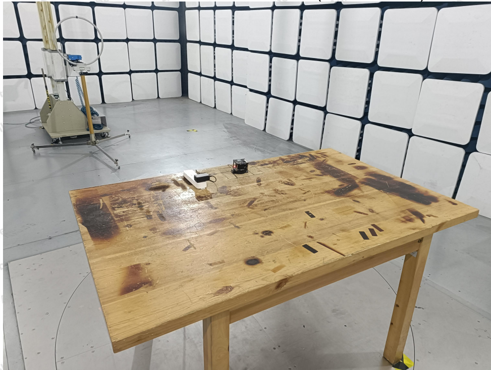
Photo of Radiation Emission Test (below 30MHz)
