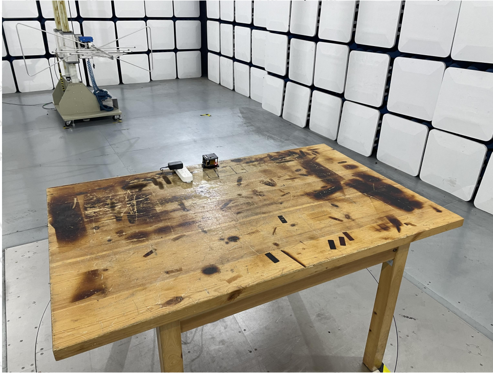
Photo of Radiation Emission Test (30MHz~1000MHz)
