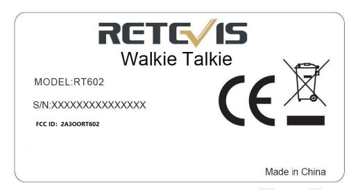
Specification: The marking shall be affixed visibly, legibly and indelibly to the radio equipment or to its data plate,
