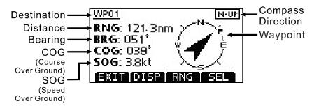
1. Press [DISP] to switch display type. Two display types are selectable.
