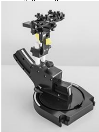
Device holder supplied by SPEAG
