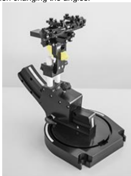
Device holder supplied by SPEAG
