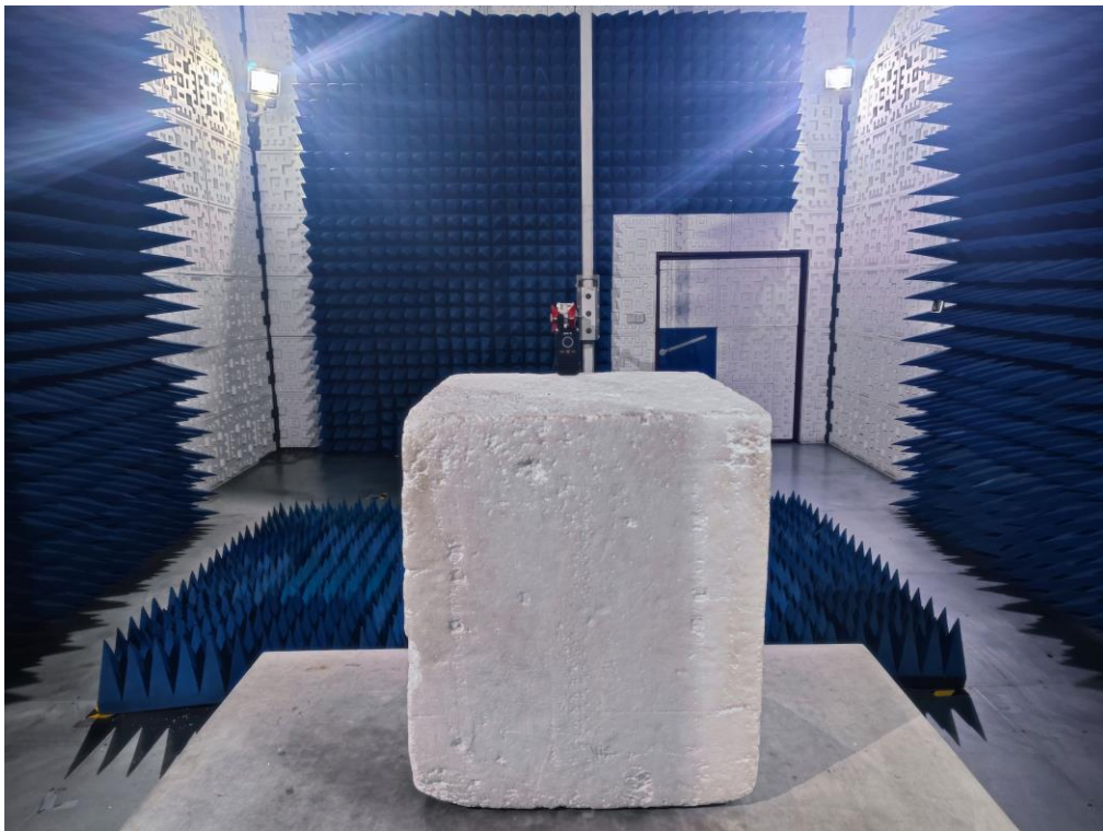
RADIATED EMISSION TEST SETUP ABOVE 1GHz
