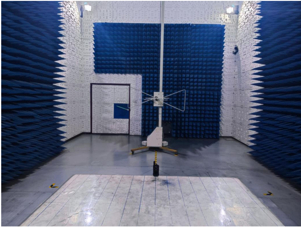
RADIATED EMISSION TEST SETUP ABOVE 1GHz
