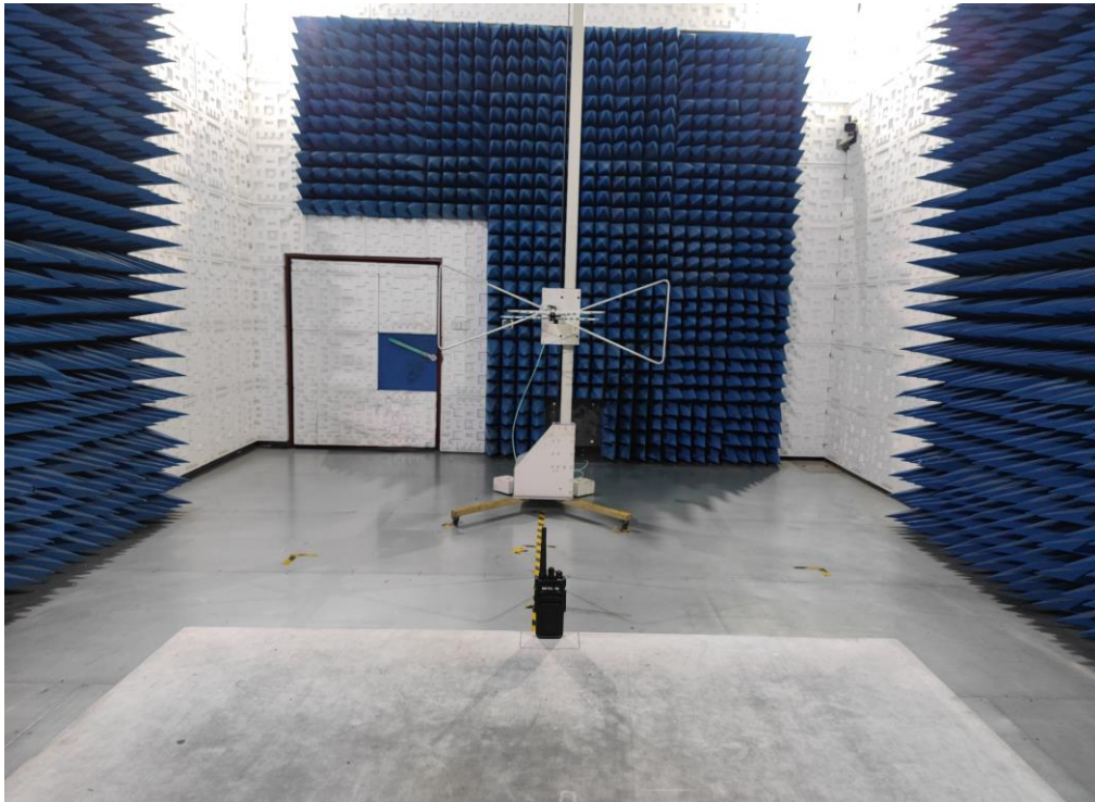
RADIATED EMISSION TEST SETUP ABOVE 1GHz
