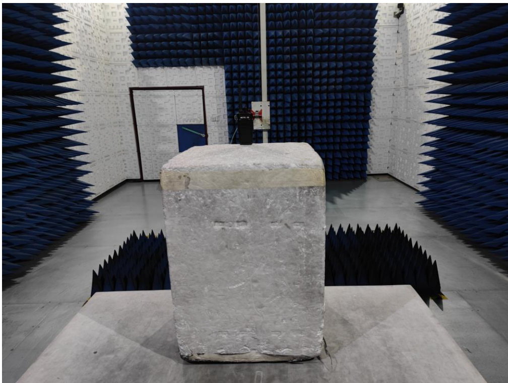
RADIATED EMISSION TEST SETUP ABOVE 1GHz
