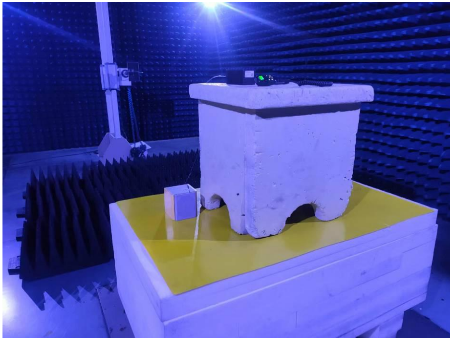
Photo of Radiated Emission Measurement (Above 1G)
