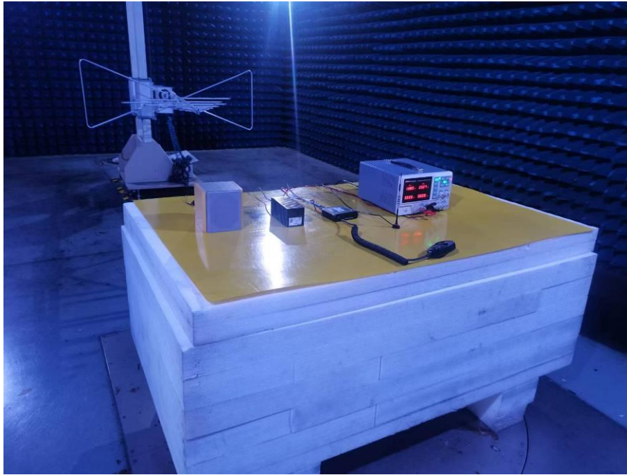
Photo of Radiated Emission Measurement (Above 1G)
