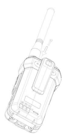
Place the belt clip to the corresponding grooves on the back of the radio, and then screw it if need. Anticlockwise turn screws to remove the belt clip.
