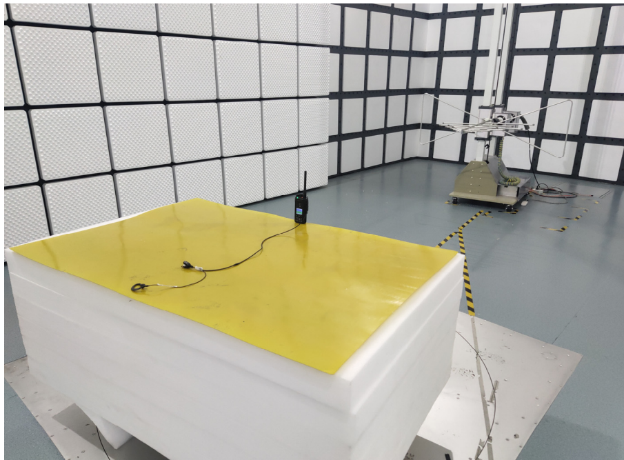
Photo of Radiated Emission Measurement (Below 1G)
