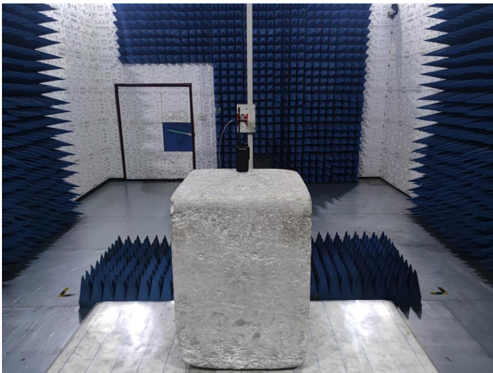
RADIATED EMISSION TEST SETUP ABOVE 1GHz
