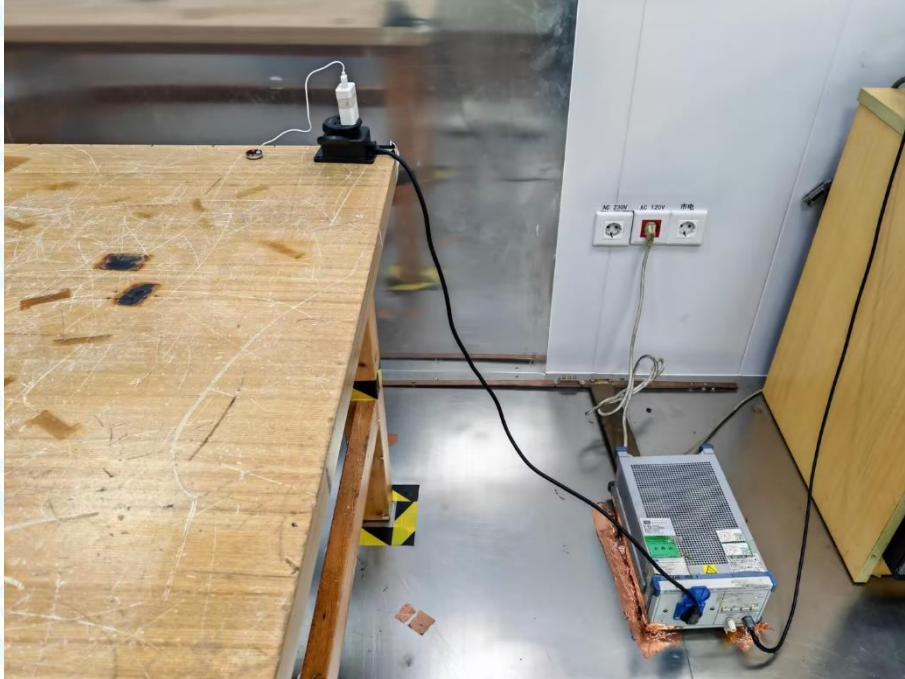
Photo of Setup for Radiated Emission (30MHz~1GHz)
