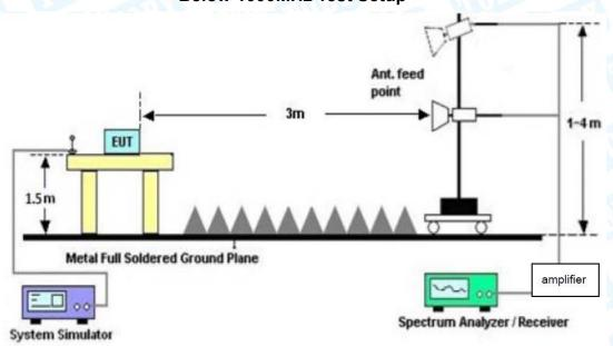
**Above 1GHz Test Setup**
