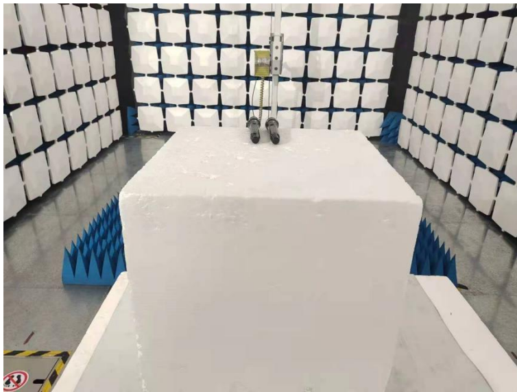
Above 1GHz for radiated emission test setup
