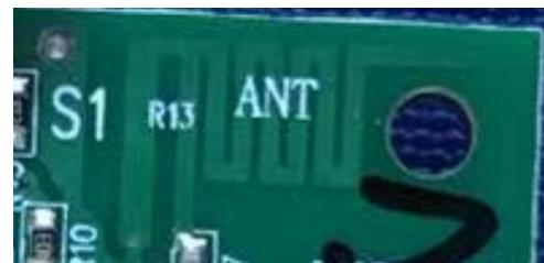
Antenna transmission frequency: 2400-2480MHz
