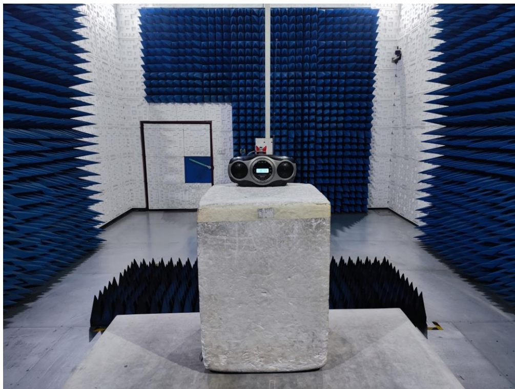
RADIATED EMISSION TEST SETUP ABOVE 1GHz
