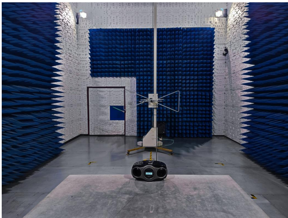
RADIATED EMISSION TEST SETUP ABOVE 1GHz
