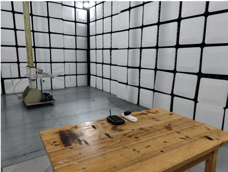
Photo of Radiation Emission Test
