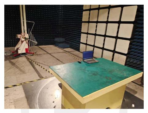
Spurious Emission Test Setup (Above 1GHz)
