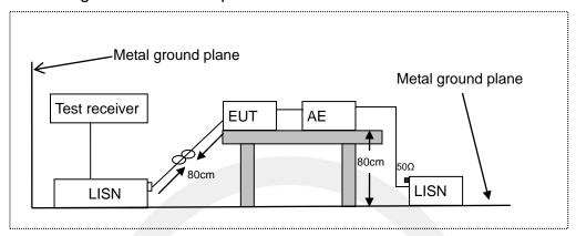
LISN: Line Impedance Stabilization Network
