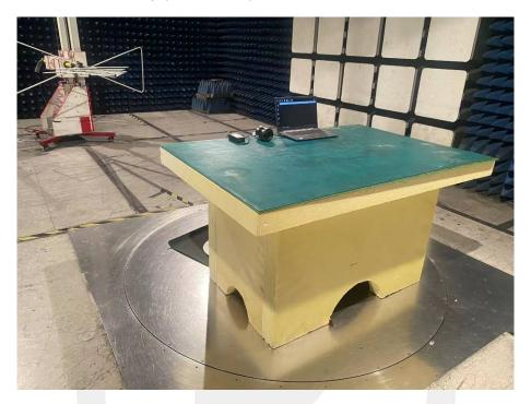
Spurious Emission Test Setup (Above 1GHz)
