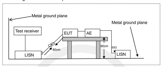
LISN: Line Impedance Stabilization Network
