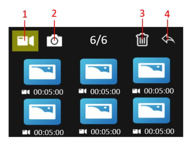
1) Video Album: Select the video album icon, press the Mode key to enter the video file selection, press the Up/Down key to select, and press the OK key to play the video. When the video is playing, you can press the "OK" key to play/pause and the key to exit. Press the Mode key to return to the album selection.
