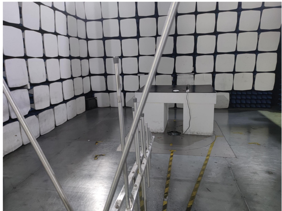
Radiation Emission Test Setup (30MHz to 1GHz)
