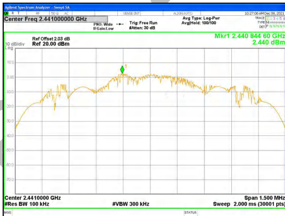
Tx. Spurious NVNT 2-DH1 2441MHz Ant1 Emission
