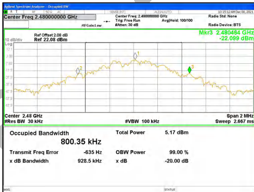
-20dB Bandwidth NVNT 2-DH1 2402MHz Ant1
