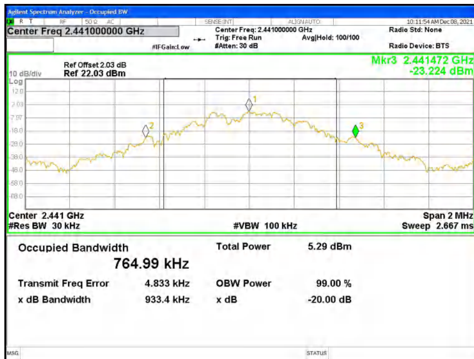
-20dB Bandwidth NVNT 1-DH1 2480MHz Ant1
