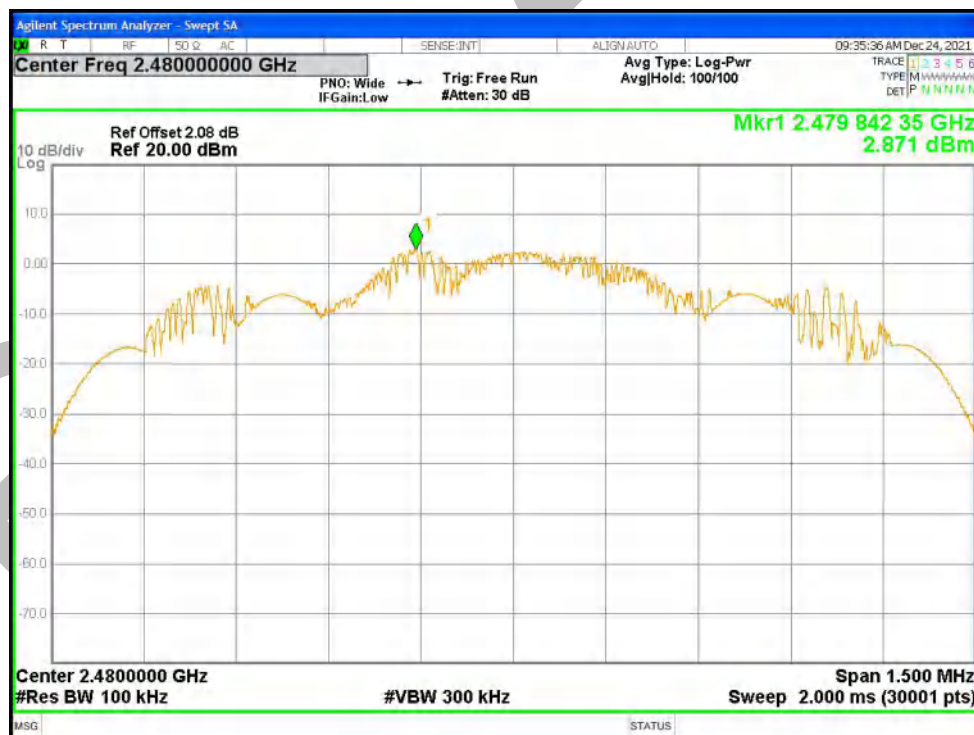
Tx. Spurious NVNT 2-DH1 2480MHz Ant1 Emission
