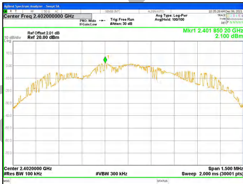
Tx. Spurious NVNT 3-DH1 2402MHz Ant1 Emission
