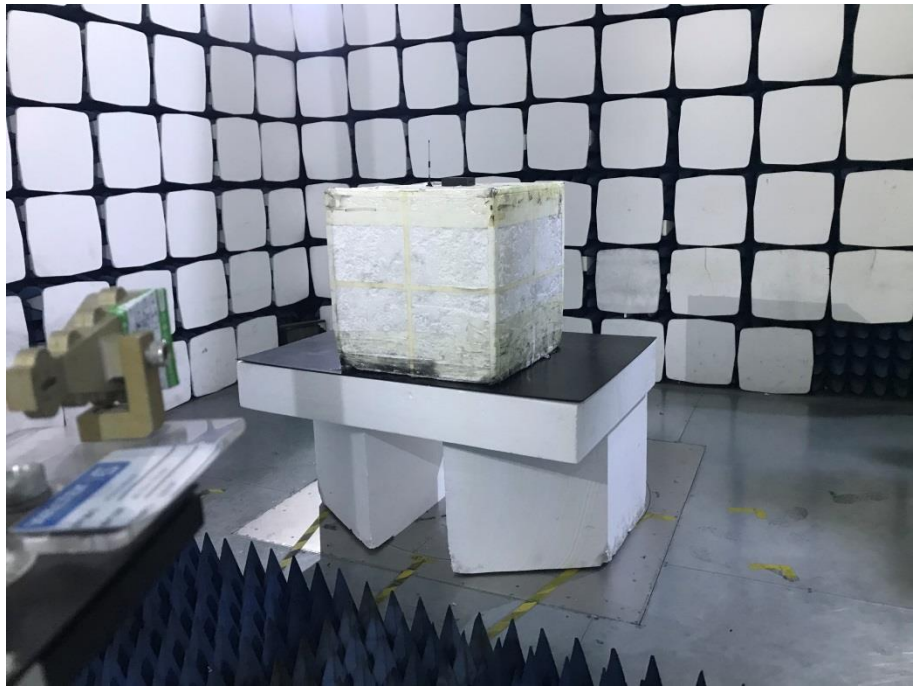
Radiation Emission Test Setup (Above 18GHz)
