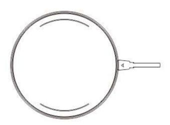
Place your phone on the wireless charger. Make sure that the phone is well located at the charging area of wireless charger. When the phone is being charged, the LED indicator will light up automatically to show charging status.
