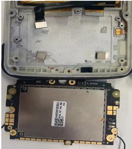
The upper motherboard is grounded to the metal frame
