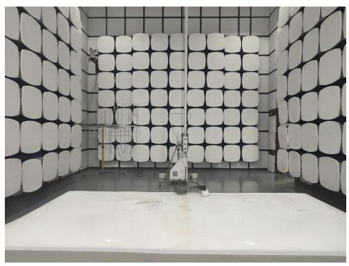
1.1. Photo of Radiated Emission test
