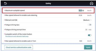
If the current speed is 2km/h below to the threshold, it will have message prompts and audible alarms which remind users the current speed is close to max limit and auto steering will be disengaged.
