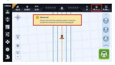
If the current speed exceeds the operators set, the auto steering will be disengaged.
