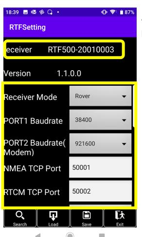
When "Smart Construction Rover 2" and Android device are connected via Bluetooth, the serial number of the connected receiver will be displayed.
