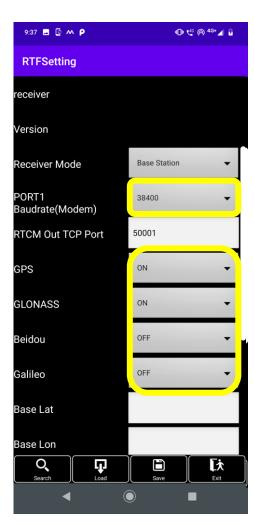
When using an external radio, "PROT1 Baudrate (Modem)" Select the baud rate of the radio used in.
