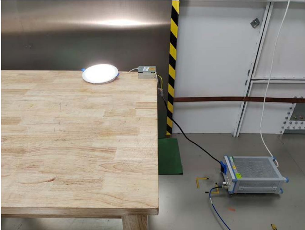
AC Power Line Conducted Emission
