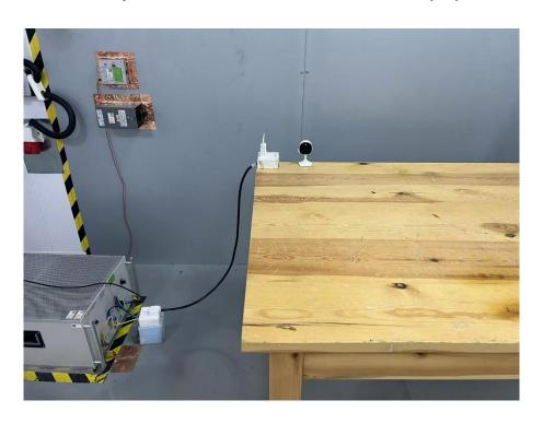
Set-up for Radiated Emission (RE), Below 1GHz
