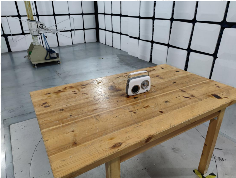
Photo of Radiation Emission Test
