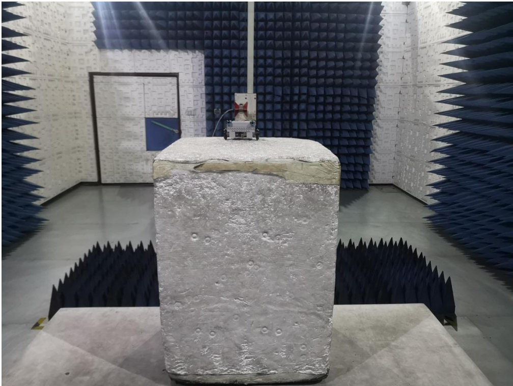
RADIATED EMISSION TEST SETUP ABOVE 1GHZ
