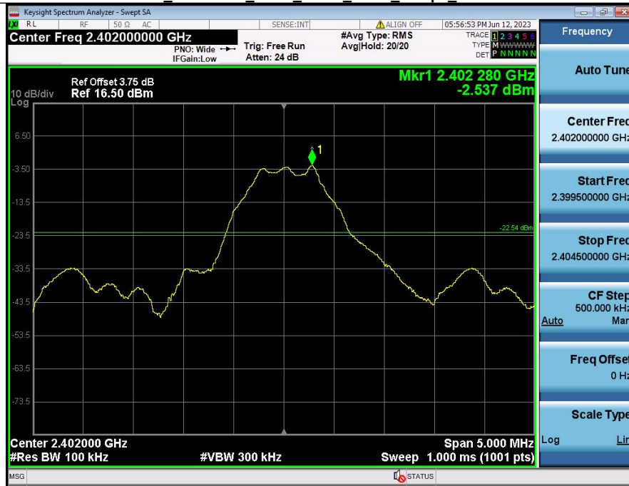
2 Spurious Emission NVNT_ANT1_1Mbps_2402
