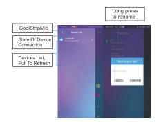
On the device page, swipe down to search for Bluetooth devices, and the searched devices will be loaded into the list. Click on any item to connect to control the device.
