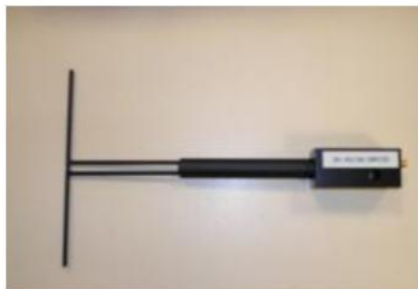
Figure 1 – Satimo COMOSAR Validation Dipole
