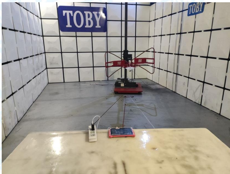
Photo of Setup for Conducted Emission
