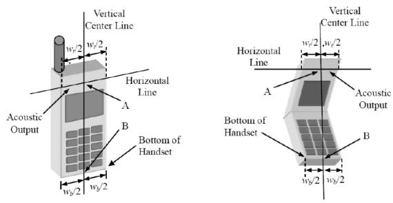
Wt Width of the handset at the level of the acoustic
