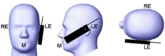
Picture 2 Cheek position of the wireless device on the left side of SAM
