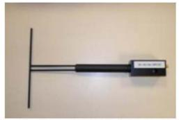
Figure 1 - Satimo COMOSAR Validation Dipole
