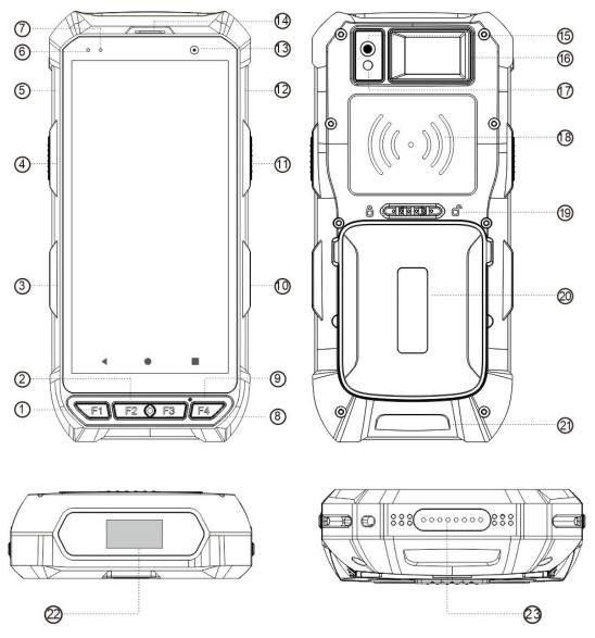
①F1 ②F2 ③Volume ④Reserved Button ⑤USB port ⑥Blue Led Indicator ⑦Red LED indicator ⑧F3 ⑨F4 ⑩Power Button ①Reserved Button ①Reserved Pogo Pin ③Front Camera ④Receiver ⑤Rear Camera ⑥Label ⑦Flashlight ⑱RFID Reading Area ⑨Battery Cover Locker ②Battery Cover ②Wrist Strap Locker ②Barcode Scan Window ③Cradle Pogo Pin Connector
