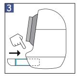
When the waste drawer is full, the POWER button light will turn red and blink slowly. The machine will stop rotating.
