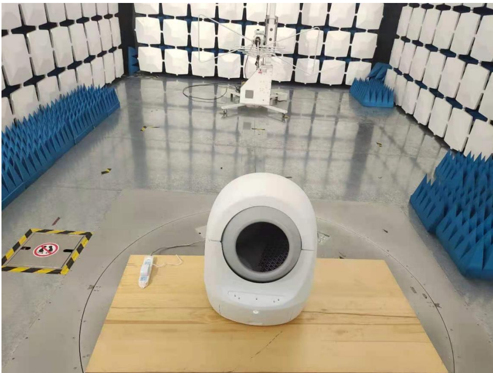
Below 1GHz for radiated emission test setup
