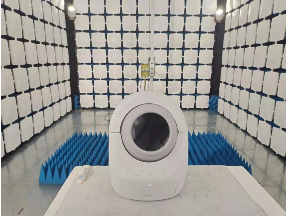
Above 1GHz for radiated emission test setup
