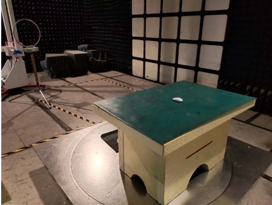
Spurious Emission Test Setup (Below 30Mhz)
