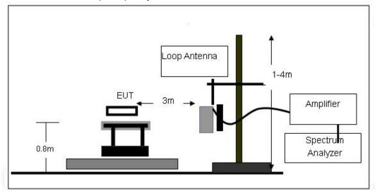
(B) Radiated Emission Test-Up Frequency 30MHz~1GHz
