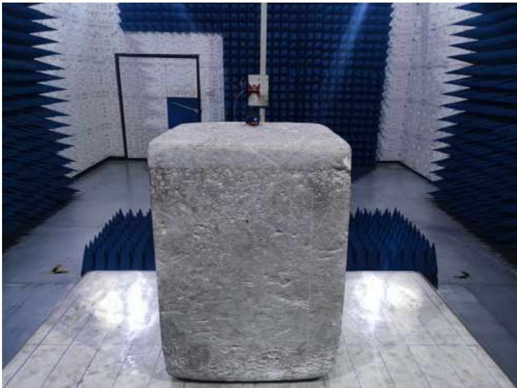
RADIATED EMISSION TEST SETUP ABOVE 1GHZ
