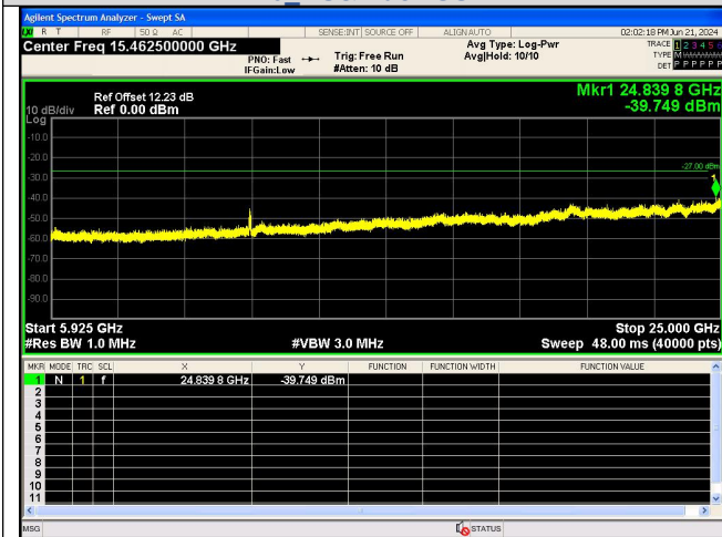
Spurious Emission:5925~25000.0 MHz IEEE 802.11ax_Channel 159_40MHz_Antenna 0_RU&Index SU
