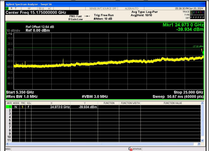
Spurious Emission:5350~25000.0 MHz IEEE 802.11n Channel 48 20MHz Antenna 0
