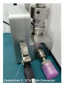
On the other end of the SCSI cable, it has individual labels on 7 Jacket cables to indicate the individual valve connection, i.e. HF => IOTHF Valve, V1 to V6 => IOT
