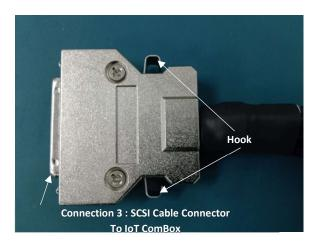
Connect SCSI Cable Connector to IoT ComBox. Please refer to photo below:
