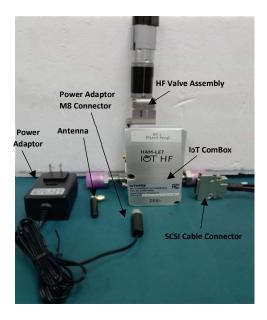
b. Connect the Antenna, Power Adaptor M8 Connector & SCSI Cable Connector to IoT ComBox. The items are in bold in the picture.
