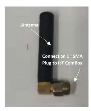
Connect the SMA plug of the right-angle antenna to the communication box per picture shown below.
