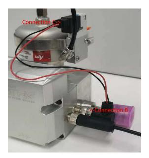
Warning! After inserting the M8 Male 4-pin plug, do remember to tighten it on the outer ring.
