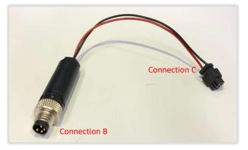
Connect the 2-pin plug into the solenoid and the M8 (Male) 4-pin to the communication
