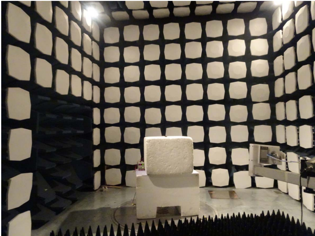
Picture 1 Radiated Emission Test Setup
